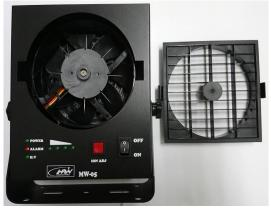
Step 3. After removing the Fan Cover, as shown in the left figure.
