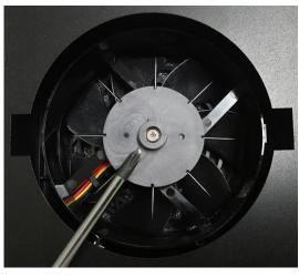
Step 4. Use a Phillips screwdriver to remove the electrode needle hub unit.
